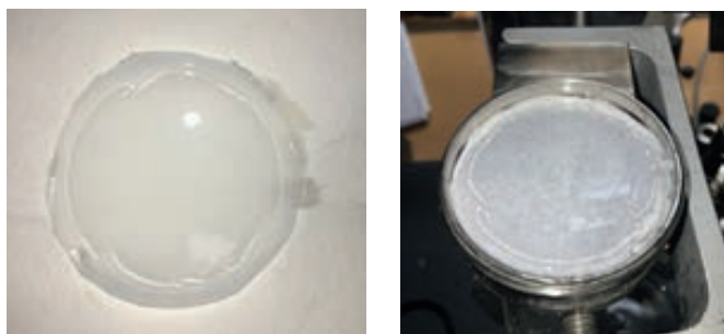
Figure 2: Image of a 0.2\mu\text{m} PVDF membrane after filtration of 1% CNC suspension at a pressure of 3.5 bar.
